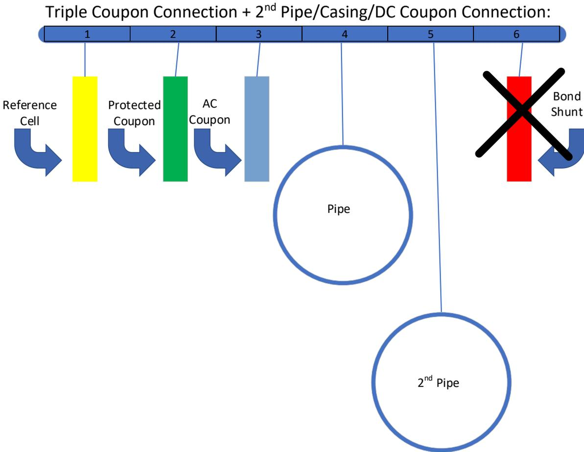
AC Coupon connection: Can read both AC and DC current. *Must be set up to read and send DC current.*
