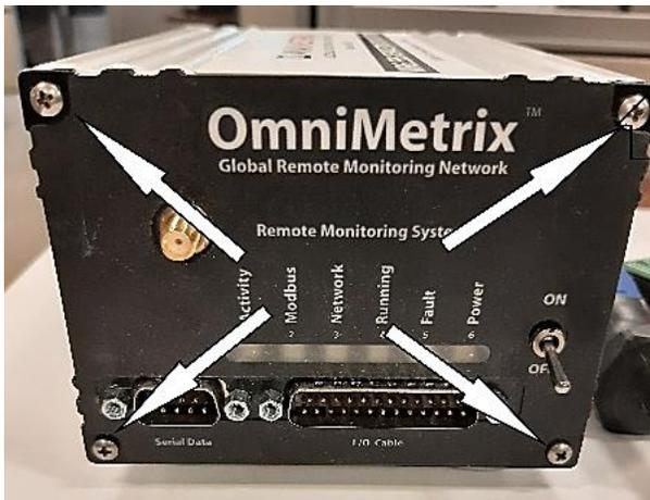
5. The front face plate slides out from the OmniMetrix case along with the main control PCB that supports the CDMA radio card. The main control PCB is aligned on the 4<sup>th</sup> notch of the case. Remember this when putting the unit back together.
