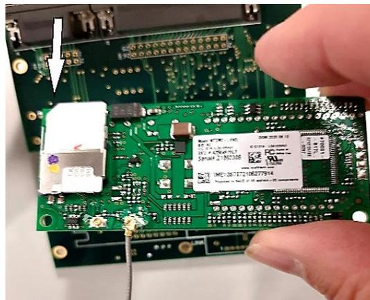
10. Gently insert the new Verizon LTE radio (pin contacts) into the same connector sockets the CDMA radio came out of. Look in between the radio board and main control board to confirm the three sets of radio pin contacts are all inserted into the existing sockets on the main controller board (All connector pins must be correctly inserted, or the LTE radio will fail to operate).
