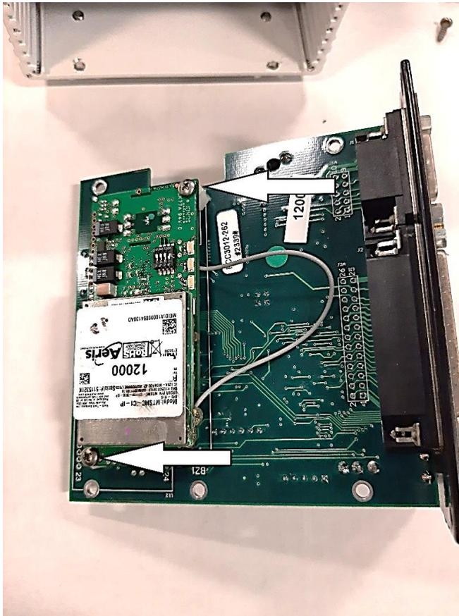
8. Once the screws have been removed, pull the radio card straight up & away from the main control PCB and **discard the CDMA radio card, old antenna connector assembly and radio card screws.**
