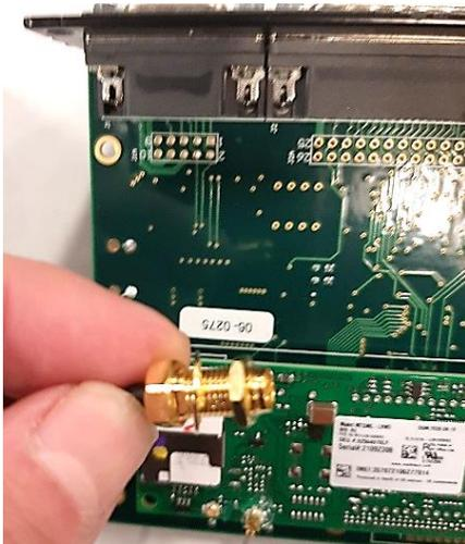
15. Turn the PCB over and route the antenna connector wire through the notch in the PCB by the SIM card of the Verizon LTE radio.
