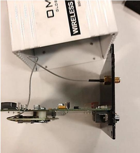
18. Slide the main control PCB/Front panel assembly back into the OmniMetrix case (remember to align the PCB with the 4<sup>th</sup> slot).
