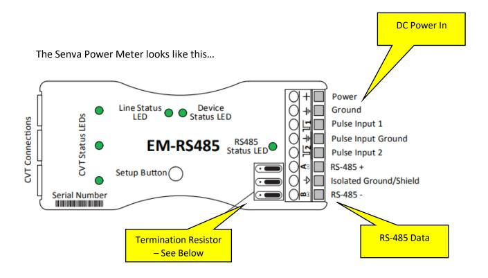
The device can mount with its own magnets, or with DIN Rail. See the Senva instructions for these details. If only one meter is used, move the center termination resistor to the left position in this view.
