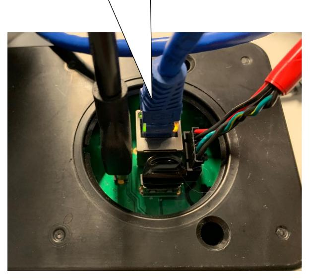
Attach the OMNI power wires, Red and Black, to generator Battery + and – respectively.
