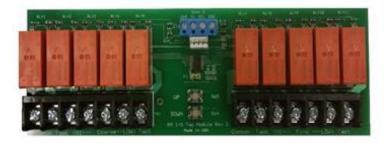
Latching relays are used to reduce current consumption.
